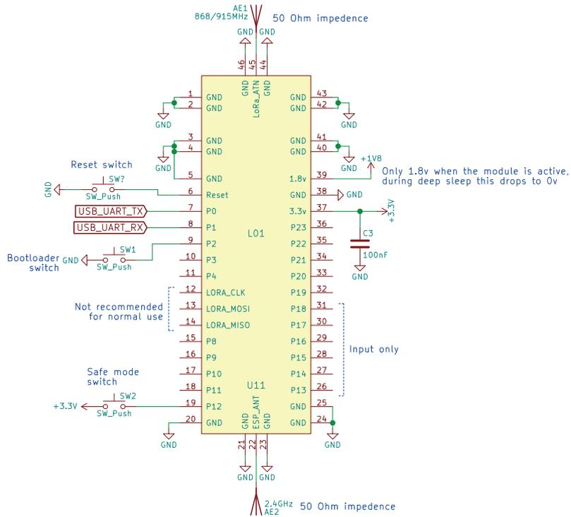
Figure 4 – Minimum required circuit
