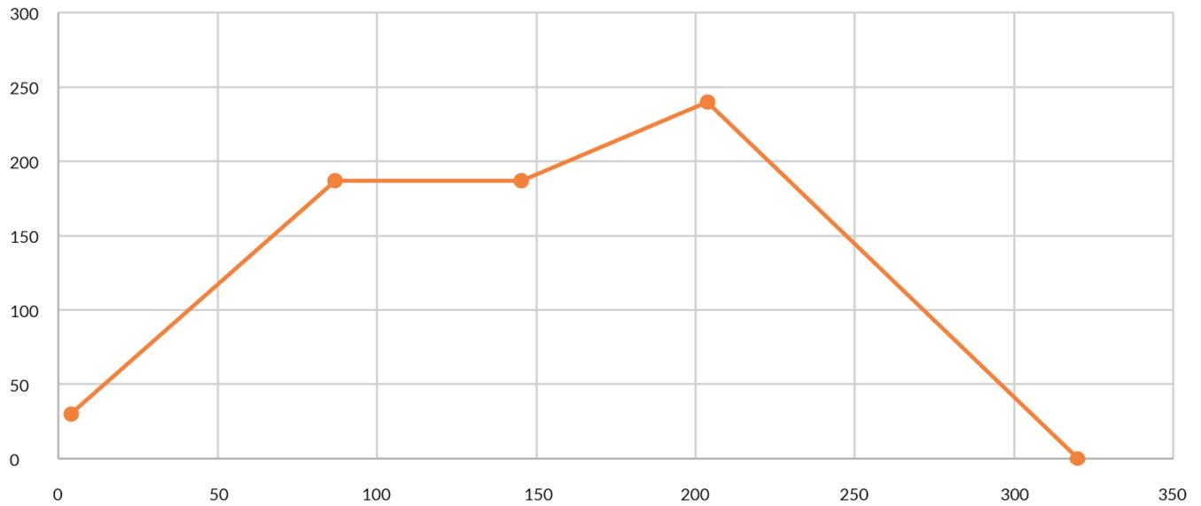
Figure 10 – Reflow soldering temperature profile
