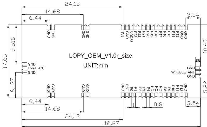
Figure 5 – Mechanical drawing (top down view)
